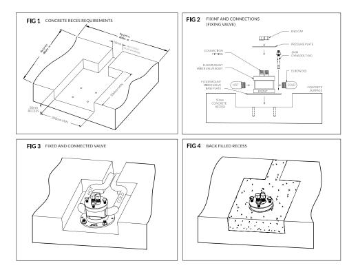
\*To install this floormount fixing valve, a 50mm step down (recess) is required in the concrete slab. The floormount fixing valve is supplied with end caps, pressure plate and fixing bolts. Leave intact until final fit off with the floormount mixer.
