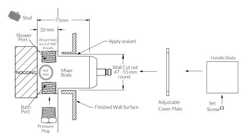
Combined wall thickness not to exceed 30mm. Wall thickness greater than 30mm, contact manufacturer prior to completing rough in.
