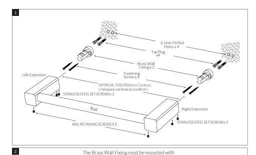
the holes in the Horizontal position as shown.
